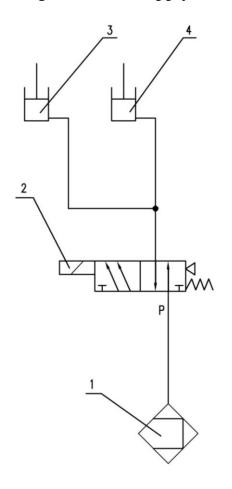
1.Air cleaner2.Solenoid Directional Valve3.Driving cylinder locking4.Assistant cylinder locking
