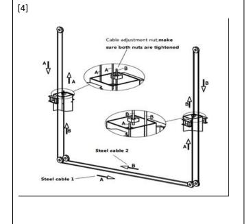
With the equalizer cables installed **raise each column and position it on the sub-frame**. Pay particular attention to the column position. Double check each column is placed in the right position.
