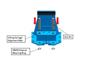
Install the arms by extending them to near full extended length. 3 stage arm will generally go to the front of a vehicle and 2 stage to the rear.
