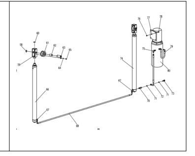
On the non-Powerside connect the long hose end to the **Cylinder Fitting** located at the base of the column.
