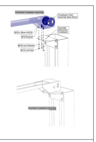
Completed installation of the Cross beam to the side columns.
