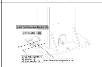
Place the Arm Extension Adapters into the arm extension adapter brackets on both the Power and Non-Powerside Posts.
