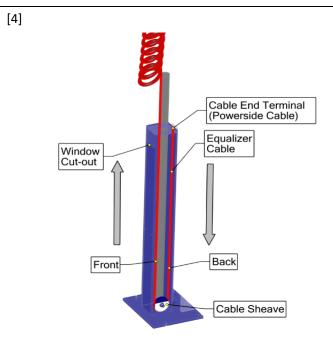
Next, remove the bottom sheave so the cable will seat, wrap cable around sheave and replace sheave with cable. Re-install after cable has been routed. [5]
