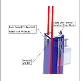
Lubricate the four inside corners of the columns with heavy duty bearing grease
