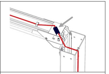
On the non-Powerside connect the long hose end to the **Cylinder Fitting** located at the base of the column.
