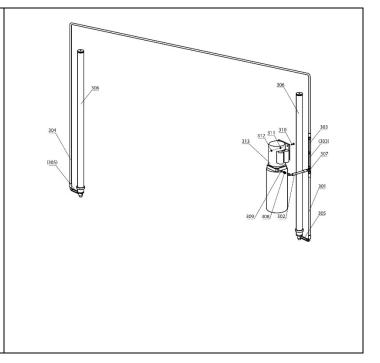
To connect the hydraulic system, first route the 9130mm (long hose) along the back of the columns and over the crossover beam assembly as shown in the diagram. This is the same for both the left and right sides.
