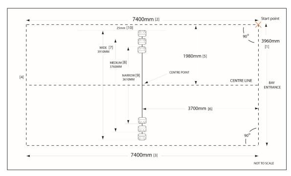
Using a measuring tape, start at one corner of the proposed area and mark a line 3960mm [1] long. Typically this is across the entrance to the bay. Working from the same start point, draw a line 90 degrees to the first line 7400mm [2] long down one side. Mark another 7200mm line [3] also at 90 degrees to the first line. At the end, draw another 3960mm [4] line that joins the two 7400 lines to complete a rectangle on the floor.
