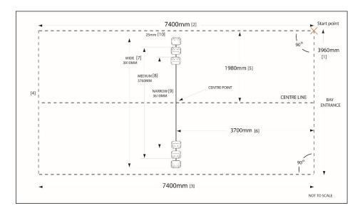
To secure the columns, work from the left-hand side first. Position the left-hand side column in the previously marked location and mark the holes using the column base plate as a guide.
